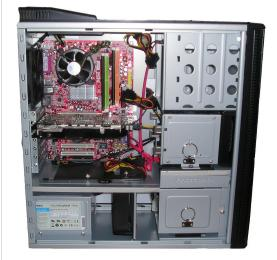
Inside a custom-built computer: the power supply at the bottom has its own cooling fan.
